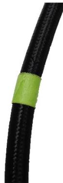
Now that we are prepared to make our cut, use a fine tooth saw or snips to cut the hose to insure a smooth final product as well as to help us as we proceed with our assembly. Secure the hose in vice jaws and begin to cut the hose ensuring to do so as straight as possible. If you are using a blade, do not force the process. Allow the blade to do the work.
