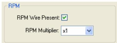
RPM Wire Present turns on the window switch function of the MAXIMIZER-3. NO check mark removes all RPM related configuration options and tells the controller to ignore RPM.
