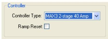
Controller type sets how the MAXIMIZER-3 will function.
