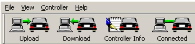
Once the software has identified the MAXIMIZER-3, the buttons will become fully visible and the connected ICON will be green.
