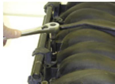
3. Now remove the factory fuel rail mounting bolts. Do not dispose of them you will be reusing them at the end of the install.
