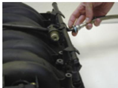
2. Use a slip-lock disconnection tool to remove your fuel line. Just disconnect the line and pull off of your fuel rail
