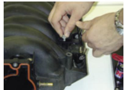
7. Now place the injectors in the fuel rail. You will need to lubricate the injector o-rings with some WD-40 or some other automotive lubricant to keep them from splitting upon reinstall. After that the NXL nozzles will need to be placed into the intake manifold. Once again be sure and lubricate their o-rings as well. Then, using the factory fuel rail mounting studs, install the NXL fuel rail mounting brackets. Make sure to leave them a little on the loose side to ease the installation.
