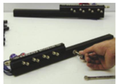
6. The rail fittings are installed in house. Then the rails are pressure checked to ensure a proper seal,. The fuel fitting must be installed next. It is located on the drivers side rail directly in the center. As with all pipe-thread fittings you must use NX thread sealer on all threads.
