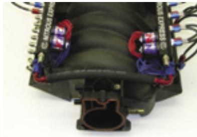
10. Before wiring up the NXL system you will need to put the fuel crossover together. First get the two Aeroquip fittings supplied in the kit, lubricate the inside of the hose ends, then slip the fittings into the hose. Be sure to butt the hose up against the coupler of the fitting. Then tighten the -AN nuts onto the NXL fuel rails and your fuel setup is complete
