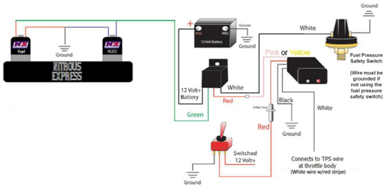
1. Mount the Master Arming Switch in a location that is within easy reach of and in plain sight of the driver.
