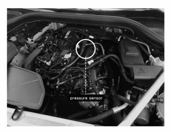
step2: Install the OEM pressure sensor on the adapter
