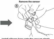
Install silicone hose onto the vacuum nipple
