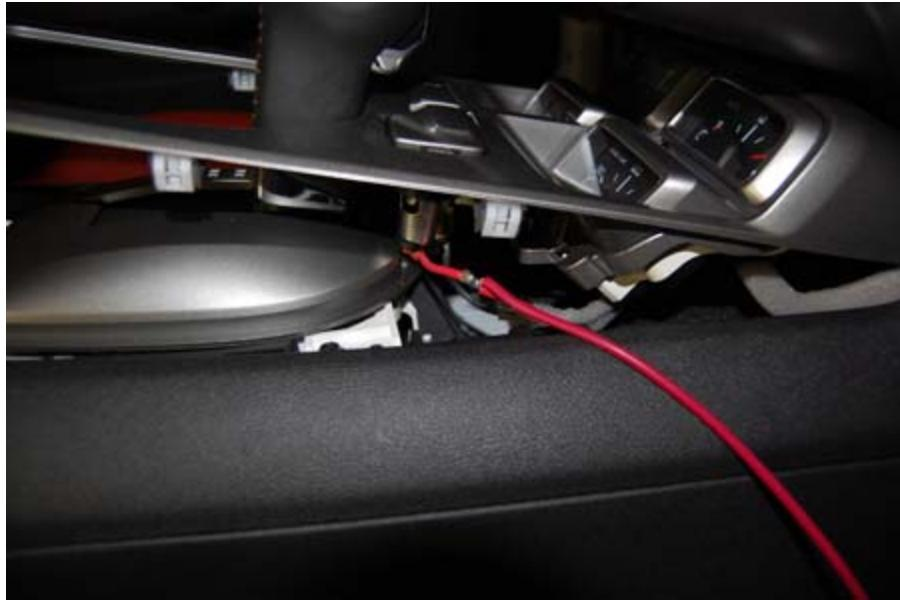
13. Choose a suitable location for the master arming switch to be mounted; the switch will need to be accessible from the driver's seat. (we chose to place our master arming switch in the A-pillar).
