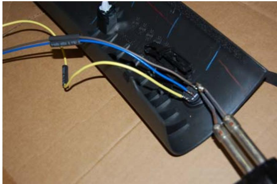
15. Connect the pink or yellow wire of the NX TPS Module to the red wire of the nitrous system relay. (this is the wire that you previously routed through the firewall)
