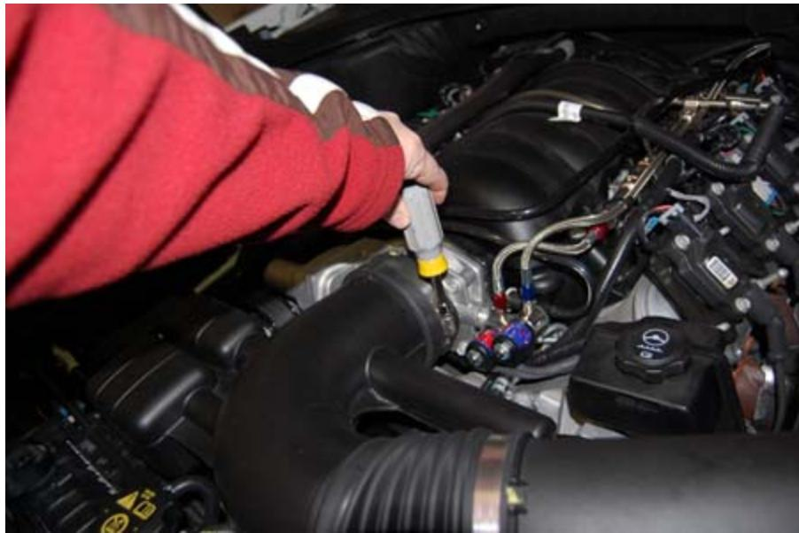
3. Unplug the harness from the throttle body and remove the four bolts that attach the throttle body to the intake manifold.
