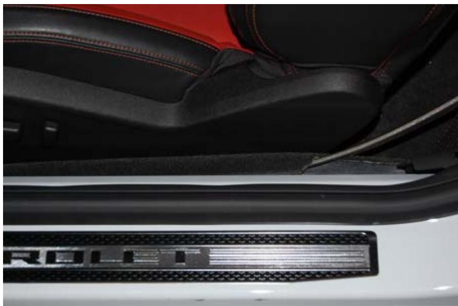
Remove the lower back seat by pulling two clips at the bottom edge of the lower seat cushion. Route the nitrous line below the back seat bottom and under the back cushion. Attach the bottle brackets to the bottle and set the bottle in the trunk with the valve facing forward.
