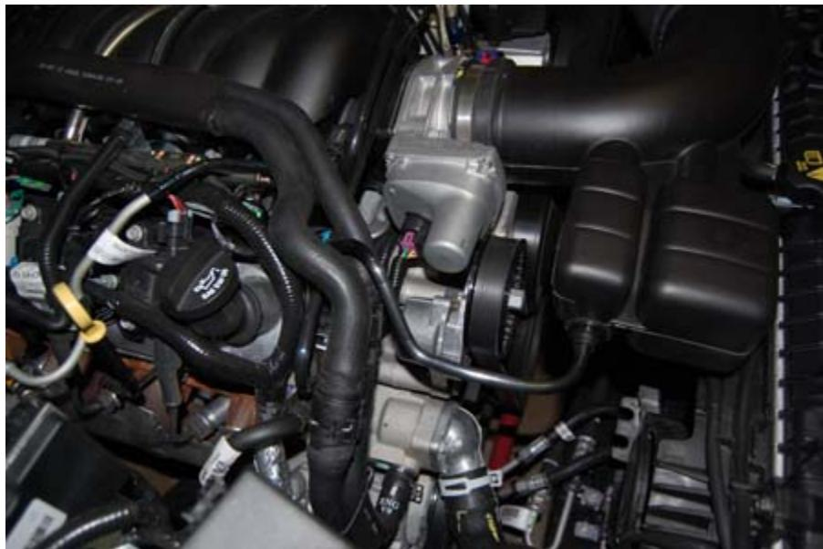
4. Apply a thin bead of silicone to the mounting flange of the throttle body.
