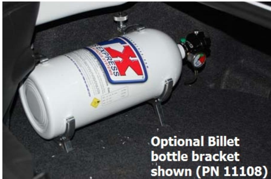
Mark the carpet through the holes in the bottle bracket. Remove the bottle and drill holes through your markings (make sure to check for wiring above and below the metal before drilling). Attach the bottle brackets using the supplied bolts, washers and nuts. Slip the bottle into the brackets and tighten. Also attach the main feed line to the bottle and slip any excess feed line below the carpet.
