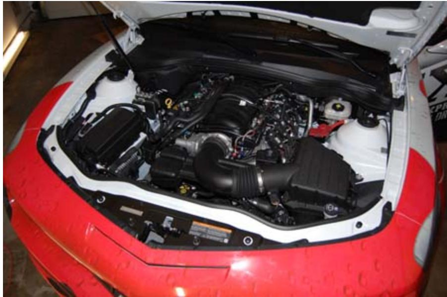
Route the nitrous line along the top of the intake, behind the insulation on the firewall, and through the firewall grommet.
