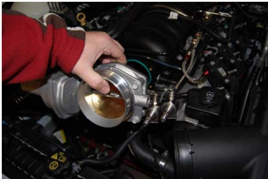
Once all four bolts are tightened, rotate the throttle blade open and verify that silicone has not protruded into the throttle body bore. If needed, wipe excess silicone out with a clean paper towel. Now plug the Throttle body harness back into the throttle body and replace the air intake tube.
