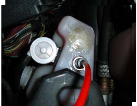
Bulkhead Fitting Installed in Washer Tank.
