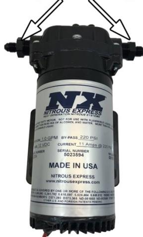
**Caution!!!** Pump must be shielded from road debris and direct tire wash. Failure to do so will result in pump failure!
