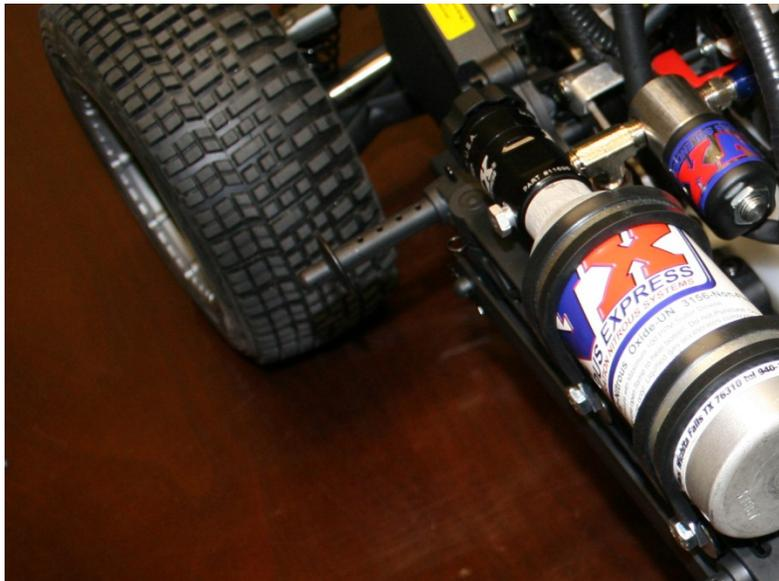
6. Install the 1/8 poly line into the push-to-connect fitting previously installed in the nitrous solenoid outlet port and route the line into the air filter. The hose should discharge toward the air filter but should not be inserted directly into it. Secure the line with zip ties.
