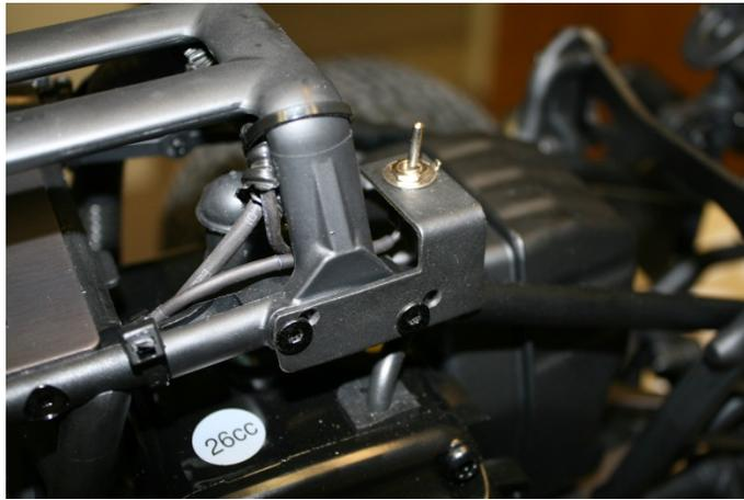
3. Now you will need to choose a location for a master arming switch. This can be anywhere that is easily accessible and so that it does not interfere with any mechanical linkages
