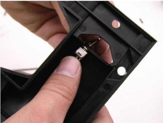
Install the supplied mini-toggle in the electronics cover.
