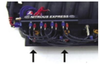
9. You may now install the nitrous and fuel lines from the rail to the nozzles. When installing start from front to back on the rail to the nozzles with the exception of the first one. If you will notice that in the third picture the front NXL nozzle on both sides of the intake, attaches to the third set of outlets. Then starting with the second one, they go from front to back, this is due to the tight radius of the hose.
