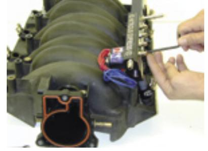
8. Once you have completed all of the before steps, it is now time to install the NXL rail. Just gently place the rail and injectors over the NXL nozzles and line them up. Press evenly and firmly until all injectors are fully seated in the nozzles. Then screw in the allen head screws through the fuel rail bracket and into the NXL fuel rail. You may finish tightening the rail mounting studs on the intake.
