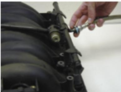
2. Use a slip-lock disconnection tool to remove your fuel line. Just disconnect the line and pull off of your fuel rail
