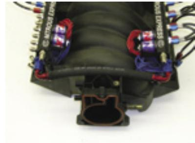
10. Before wiring up the NXL system you will need to put the fuel crossover together. First get the two Aeroquip fittings supplied in the kit, lubricate the inside of the hose ends, then slip the fittings into the hose. Be sure to butt the hose up against the coupler of the fitting. Then tighten the -AN nuts onto the NXL fuel rails and your fuel setup is complete
