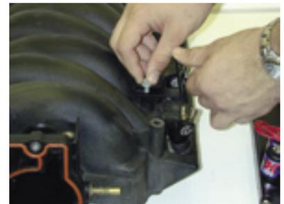
7. Now place the injectors in the fuel rail. You will need to lubricate the injector o-rings with some WD-40 or some other automotive lubricant to keep them from splitting upon reinstall. After that the NXL nozzles will need to be placed into the intake manifold. Once again be sure and lubricate their o-rings as well. Then, using the factory fuel rail mounting studs, install the NXL fuel rail mounting brackets. Make sure to leave them a little on the loose side to ease the installation.
