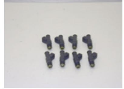
5. Flip injector rail over. This will allow you to remove injector lock clips. Once you have removed the clips take the injectors off of the fuel rail. Then inspect both o-rings on every injector. If the o-ring has the slightest tear or cut, replace before reinstalling.
