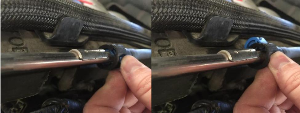
3. Assemble the 16185 Fuel Rail Adapter using Red or Blue NX Sealant. Push the 16185 Fuel Rail Adapter up onto the fuel rail until it clicks into place. Snap the fuel line over the 16185 Adapter.
