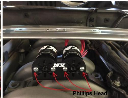
5. Using NX Red/Blue Sealant, screw the 1/8npt to 4an fitting into the "N2O In", and the other 1/8npt to 4an into the "Fuel In". The one with the filter screen goes in the nitrous solenoid.
