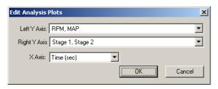
The X and Y-axis can be customized to display any combination of. This is done by selecting the items from the pull-down menus for each axis. For example, viewing EGO on the Y-axis and RPM on the X-axis will display your air-fuel ratio over your RPM range. The **acceleration plot** indicates how fast the RPM was increasing which can be used to compare performance from one run to the next as well as analyzing wheel spin or other conditions.
