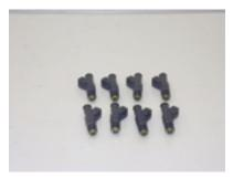
5. Flip injector rail over. This will allow you to remove injector lock clips. Once you have removed the clips take the injectors off of the fuel rail. Then inspect both o-rings on every injector. If the o-ring has the slightest tear or cut, replace before reinstalling.
