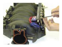
8. Once you have completed all of the before steps, it is now time to install the NXL rail. Just gently place the rail and injectors over the NXL nozzles and line them up. Press evenly and firmly until all injectors are fully seated in the nozzles. Then screw in the allen head screws through the fuel rail bracket and into the NXL fuel rail. You may finish tightening the rail mounting studs on the intake.
