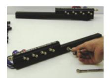
6. The rail fittings are installed in house. Then the rails are pressure checked to ensure a proper seal,. The fuel fitting must be installed next. It is located on the drivers side rail directly in the center. As with all pipe-thread fittings you must use NX thread sealer on all threads.
