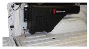
Prepare the bed rail for reservoir installation. Remove any other hardware such as tonneau cover bed rails.
