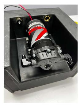
**Step 4** Install the supplied 4an line from the tanks outlet to the pumps inlet. Finally mount your tank in the desired location and enjoy your Snow Performance Water/Methanol System.
